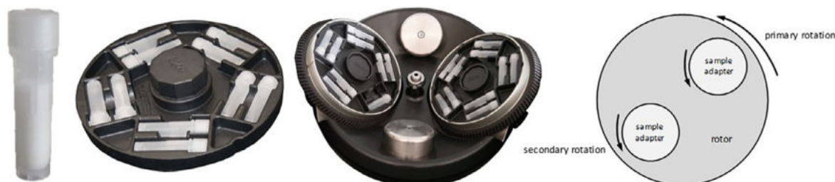
Fig. 2. 2 DC-Twist-Top-Vial (PP), sample adapter (middle) and rotor including sample adapters (right) of dual centrifuge.
