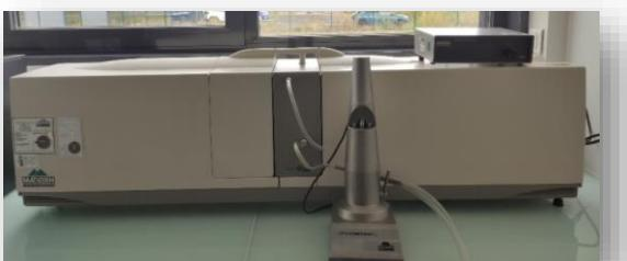
Particle size analysis using laser diffraction particle size analyzer (Mastersizer 2000, Hydro 2000SM Malvern)
