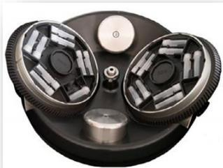
**Nanomilling** using dual centrifugation, 1500 rpm, 90min, 4°C (Zentrimix 380R, Hettich)
